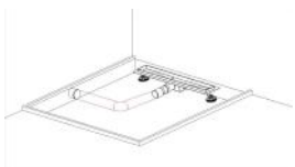
4. Install the water pipes
